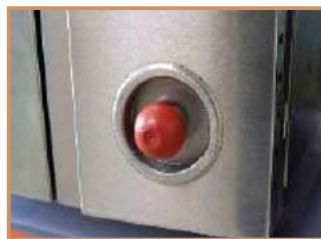
Manual drain valve for emptying the water tank
