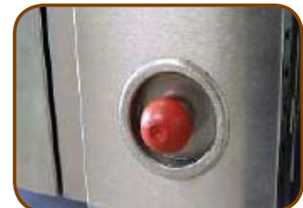
Manual drain valve for emptying the water tank
